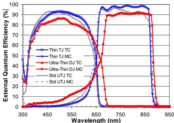
Fig. 2 Comparison of thin TJ cells, ultra-thin DJ cells, and UTJ cells external quantum efficiency performance.
