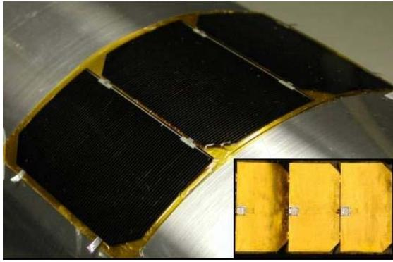
Fig. 5 A prototype thin-cell coupon rested on a 95-mm radius cylinder.
