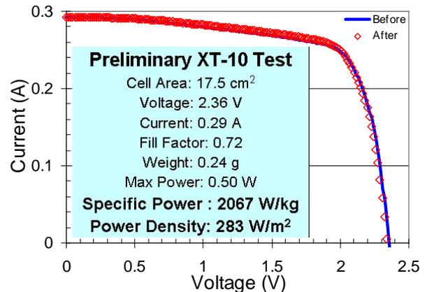
Fig. 8 Illuminated I-V characteristic of an ultra-thin DJ cell before and after flex.
