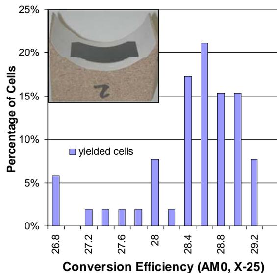
Fig. 4 Efficiency distribution of 50 large-area thin, TJ cells.
