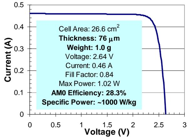
Fig. 3 Illuminated I-V data of prototype thin-cell coupons with (#1) and without (#2) bypass diodes.
