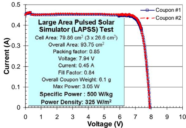
Fig. 6 Illuminated I-V data of prototype thin-cell coupons with (#1) and without (#2) bypass diodes.
