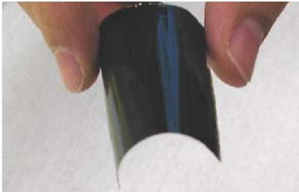
Fig. 9 Flexing of a large-area ultra-thin DJ cell.
