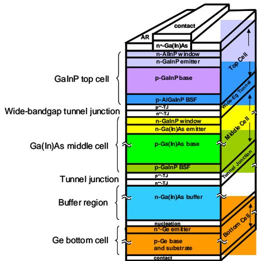
Fig. 1 Cross-sectional schematic of a thin TJ cell structure.
