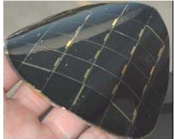
Fig. 7 Sixteen 2.25-cm<sup>2</sup> ultra-thin DJ cells in 4" wafer format.
