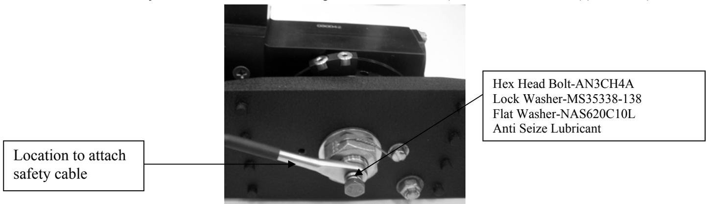
**Figure 17 Install Safety Cable**
