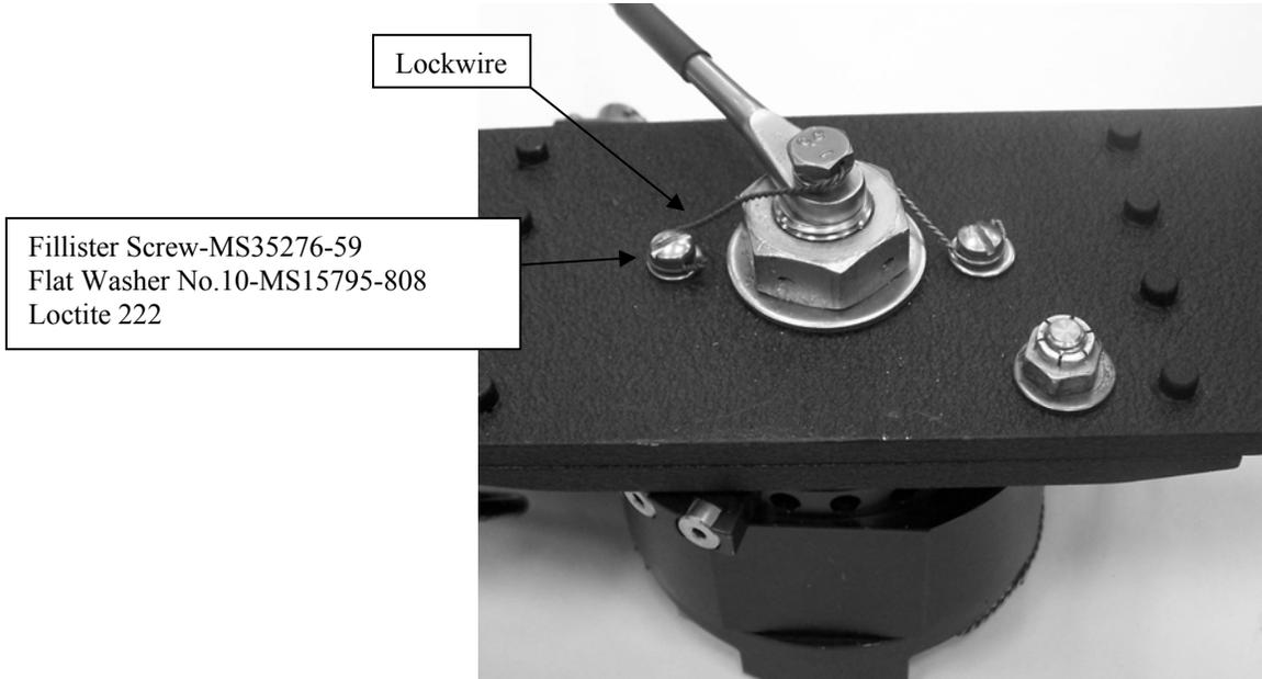
**Figure 19 Install Lock Wire**
