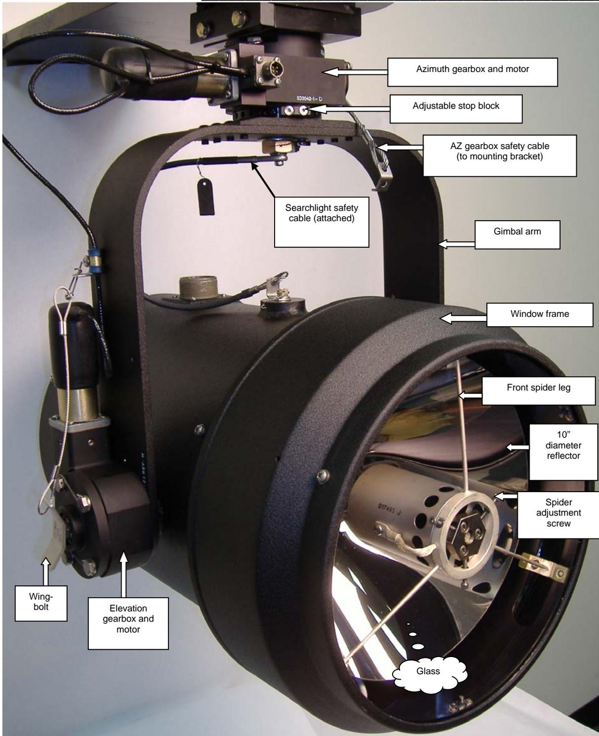
Figure 13 Searchlight Mounted in Gimbal (Current Configuration)
