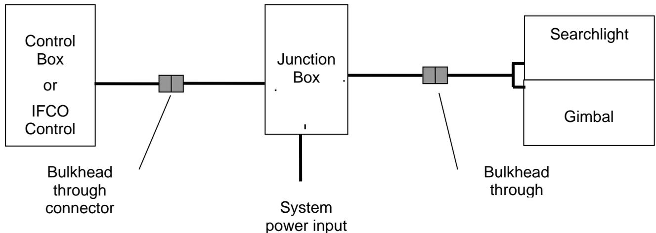
**Figure 7 Overview of Connections between SX-16 Nightsun® Components**
