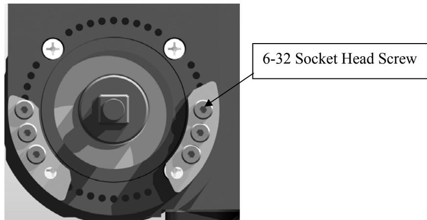
**Figure 12 Elevation Mechanical Stops**
