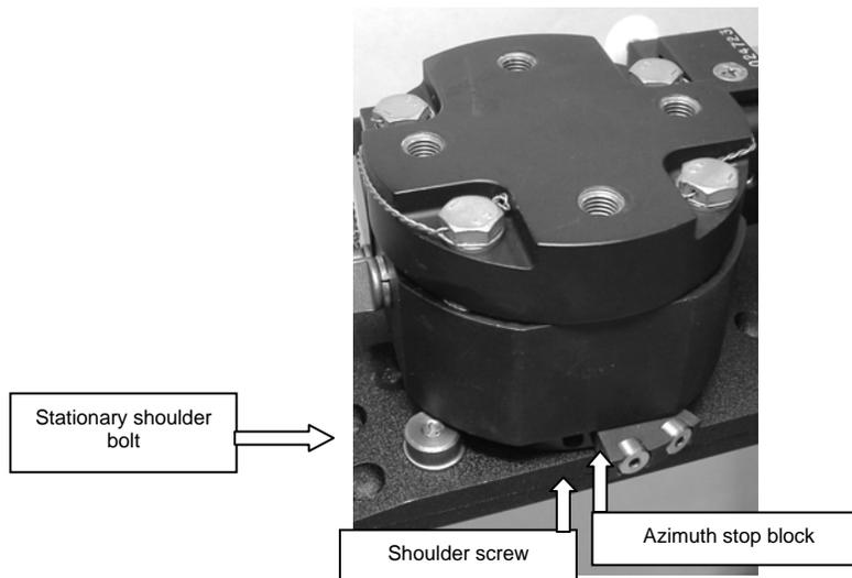
**Figure 11 Current Azimuth Stop Configuration (Shown on doubler type Gimbal Arm)**
