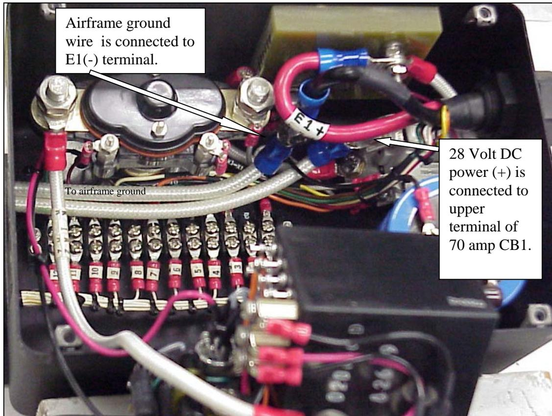
**Figure 5. Step 4. CONNECTIONS OF AIRCRAFT POWER (+) AND (-) CABLES INTO JUNCTION BOX.** Positive input power is connected to upper terminal of 70 amp circuit breaker. Negative input power (i.e. airframe ground) is connected to E1(-) terminal, on top of searchlight power (-) wire.
