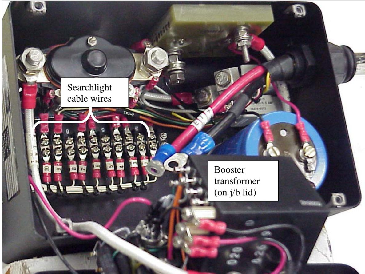
**Figure 2 Step 2. SEARCHLIGHT CABLE CONTROL WIRE CONNECTIONS** to terminal strip TB1. Numbered AWG 20 wires are connected to the row of screws across from control cable wire connections. Wire numbers correspond to those on control cable wires. (booster transformer in foreground)
