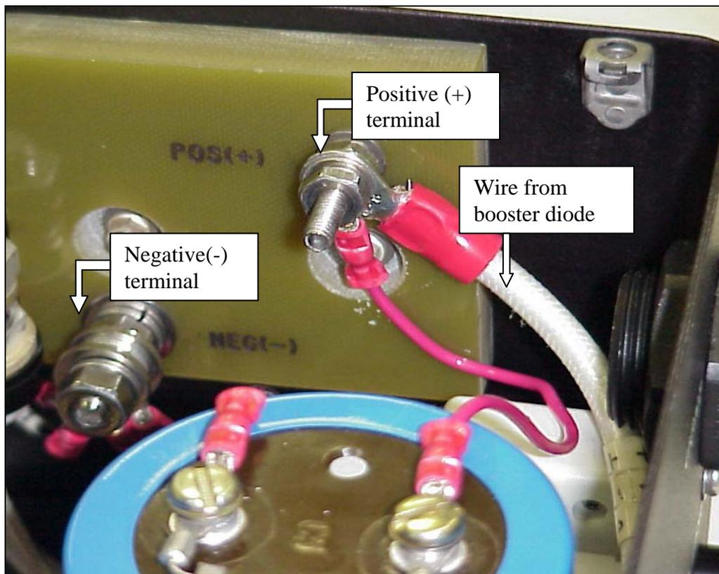
**Figure 3. CLOSE UP VIEW OF E1 TERMINAL BLOCK.** Negative terminal at bottom has 1/4-20 threads. The positive terminal at top has 10-32 threads. The wires (shown) attached to the positive terminal are from the capacitor and the booster. They remain in **SPECTROLAB NIGHTSUN® and STARBURST® SEARCHLIGHTS**
