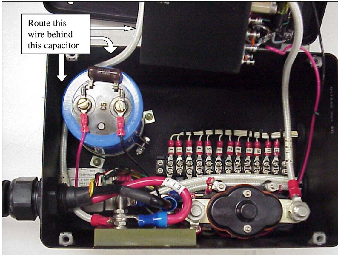
**Figure 6. Step 5. FINAL ROUTING OF WIRES IN JUNCTION BOX BEFORE CLOSING COVER.** Routing the (+) wire from the top of the booster diode behind the large blue capacitor is necessary to prevent damaging the wire or its insulation. Make one final verification that all wires are properly placed and all terminals are tight before replacing cover.
