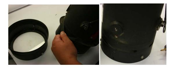
4. Secure the Front Window Assembly to the Searchlight Housing with 3 screws previously removed.
