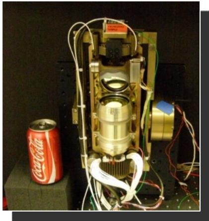
Figure 11 The compact LADAR system integrated with the Spectrolab Gen-II LADAR camera by Boeing DES.
