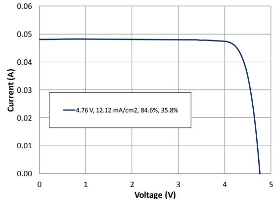
Fig. 1: Illuminated I-V curve for a 4-cm<sup>2</sup>, 35.8%-efficient space direct-bonded 5J cell, measured at 1-sun, AM0, 25°C at NREL.
