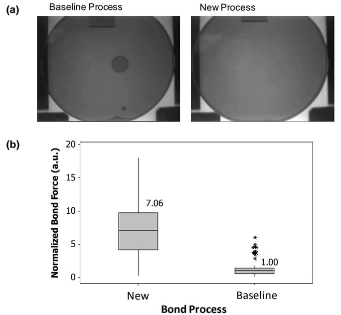
Fig. 6: Comparison of (a) IR bond images (b) normalized bond pull force between baseline and new bond processes.
