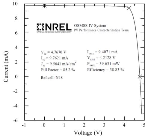
Fig. 3: Illuminated IV curve for a record 38.8%-efficient terrestrial 1cm<sup>2</sup> 5J direct bonded cell. The cell was measured at 1 sun under the AM1.5G spectrum, 25°C at NREL.
