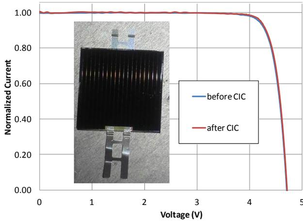
Fig. 2: Illuminated I-V curve for a 4-cm<sup>2</sup> cell before and after the CIC process. Inset shows a picture of a direct-bonded 5J CIC. Current is normalized for the purpose of comparison.
