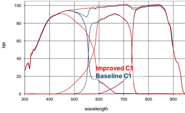
Fig. 5: IQE for GaAs T3J cells. Red and blue curves correspond to the IQE of the T3J with improved and baseline C1 growth conditions, respectively.
