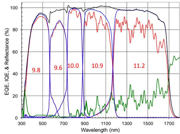
Fig. 4: EQE, IQE and reflectance curves for record SBT 5J cell. EQE, IQE, and reflectance are given by the blue, red, and green curves respectively. Cumulative IQE, the total obtained by summing the IQE from every subcell at each wavelength, is given by the black curve. Integrated  $J_{sc}$  values calculated from EQE for each cell are shown by the red numbers.
