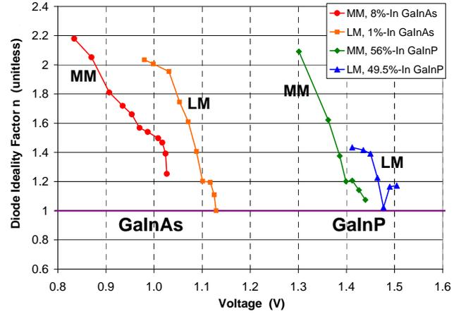
Fig. 7. Diode ideality factor  $n$  as a function of voltage for MM and LM solar cells.
