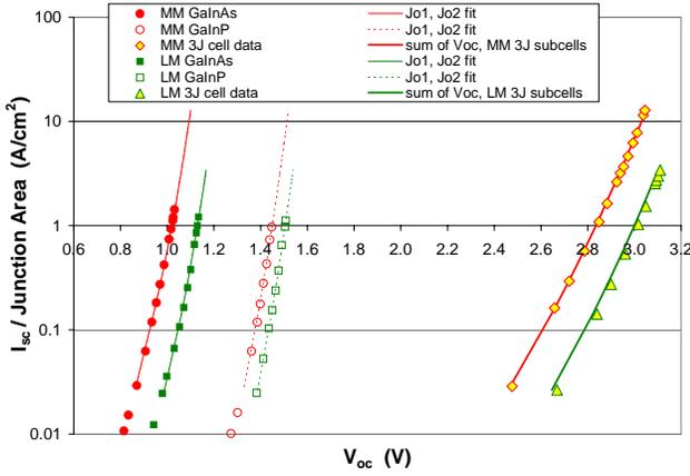
Fig. 6.  $J_{sc}$  vs.  $V_{oc}$  plots at varying intensities for metamorphic and lattice-matched GaInAs, GaInP, and 3-junction cells, and fits to the data using extracted  $J_{o1}$  and  $J_{o2}$  values.
