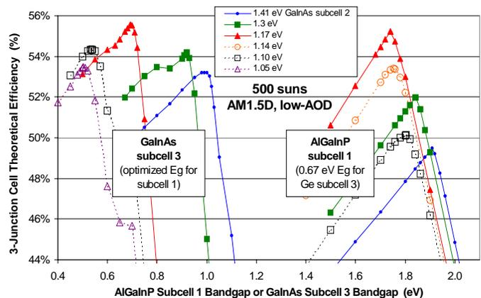
Fig. 1. Calculated ideal efficiency of 3-junction solar cells as a function of subcell 1, 2, and 3 bandgaps.
