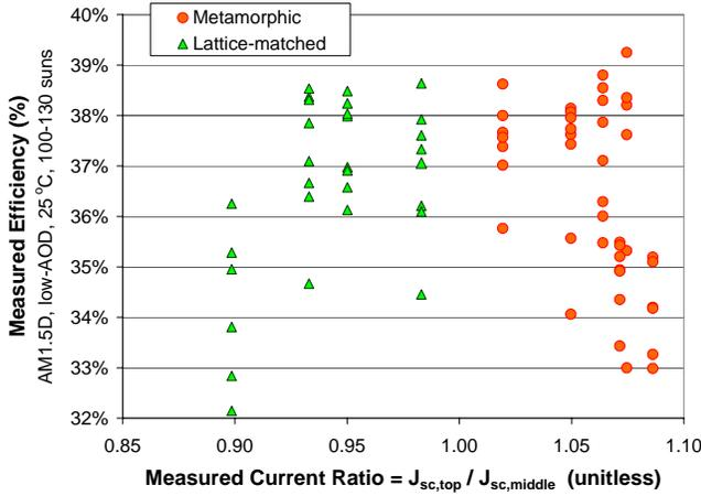
Fig. 4. Multijunction terrestrial concentrator cell efficiency at 100-130 suns, tested at Spectrolab using NREL-calibrated reference cells, plotted vs. current ratio.
