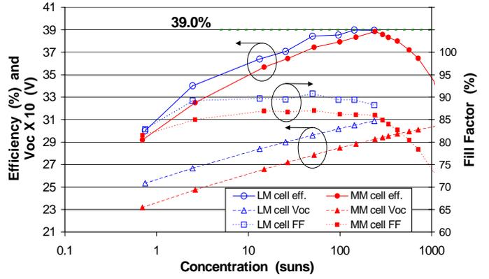
Fig. 5. Dependence of efficiency,  $V_{oc}$ , and FF on solar concentration ratio for record-efficiency metamorphic and lattice-matched 3-junction cells.
