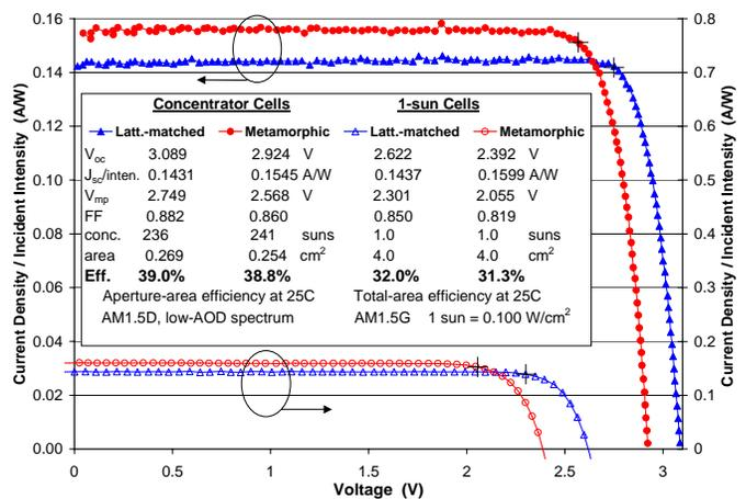
Fig. 3. Light I-V curves for record efficiency metamorphic cell with 38.8% efficiency, and record efficiency lattice-matched cell with 39.0%, under the concentrated AM1.5D, low-AOD terrestrial solar spectrum. Record efficiency MM and LM one-sun cells are also shown for comparison.
