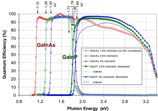
Fig. 2. Measured quantum efficiency for metamorphic and lattice-matched GaInAs and GaInP subcells. Both disordered and ordered cases for the group-III sublattice of GaInP are shown.
