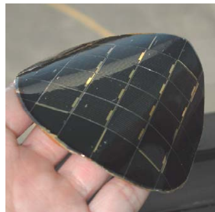
Fig. 13. Sixteen 1.5 cm x 1.5 cm ultra-thin solar cells on 50- \mu\text{m} -thick kapton sheet.
