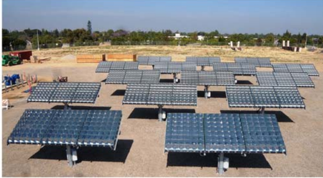
Figure 5. Boeing/SES test system with C4MJ cells installed
