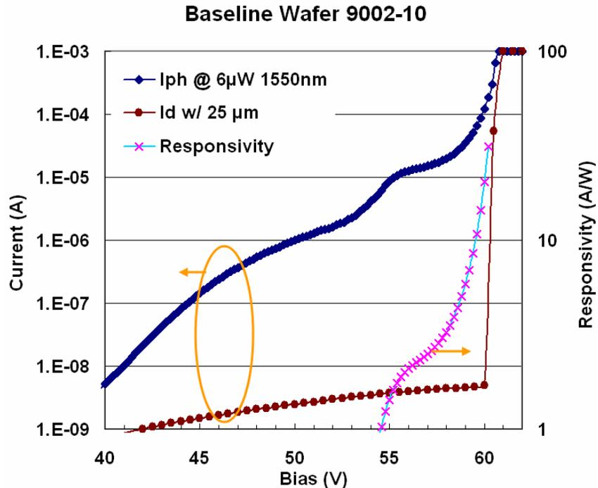
Figure 2 The DC current-voltage and responsivity-voltage characteristics of a Spectrolab 1.55  $\mu\text{m}$  GM APD.
