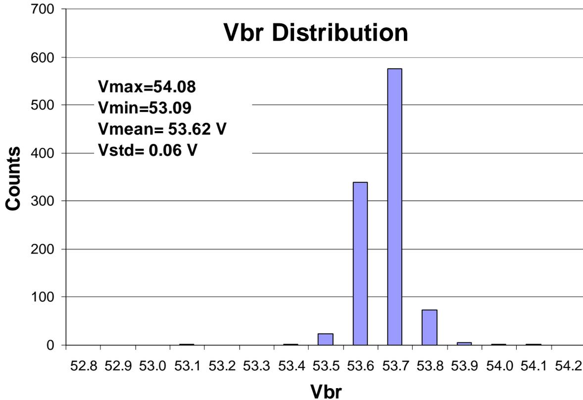
Figure 7 The histogram of the breakdown voltage of a 32x32 1.55  $\mu\text{m}$  GM-APD at room temperature.
