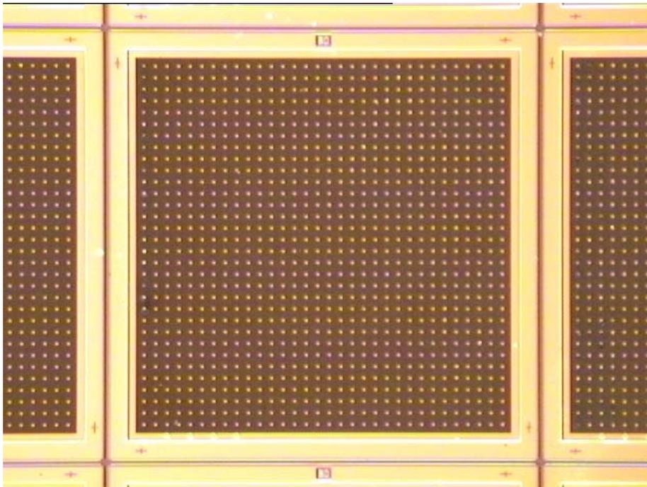
Figure 6 The fabricated 32x32 GM-APD arrays.
