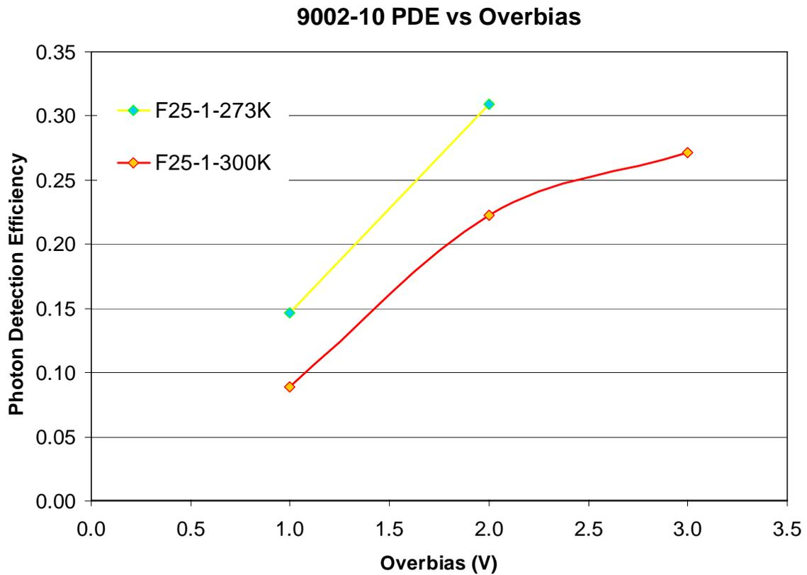
Figure 4 The PDE vs overbias at room temperature and 0°C versus overbias. The PDE was measured at 1.55  $\mu\text{m}$ .
