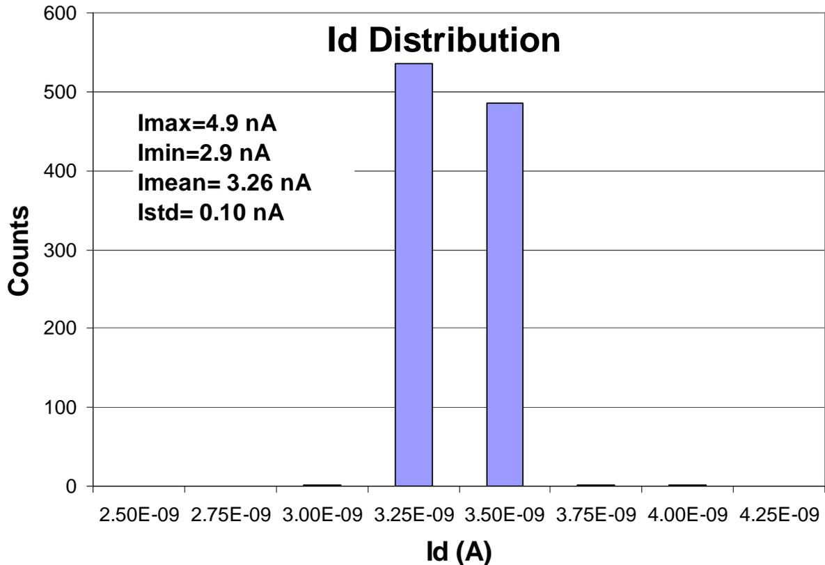
Figure 8 The histogram of the dark current before breakdown of a 32x32 1.55  $\mu\text{m}$  GM-APD at room temperature.
