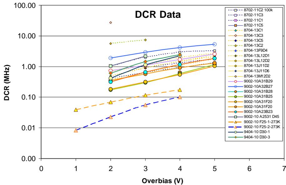
Figure 3 The DCR at room temperature and 0°C versus overbias characteristics taken on two types of GM-APDs. The 8702 and 8704 APDs were InGaAsP/InP APDs optimized for 1.06 μm, and their curves are shown with dotted lines and smaller markers. The 9002 and 9404 series APDs are sensitive at 1.55 μm and yet display a very low DCR even at room temperature. They are illustrated with solid lines. The DCRs of the 9002 APDs at 0°C are shown with dash lines.
