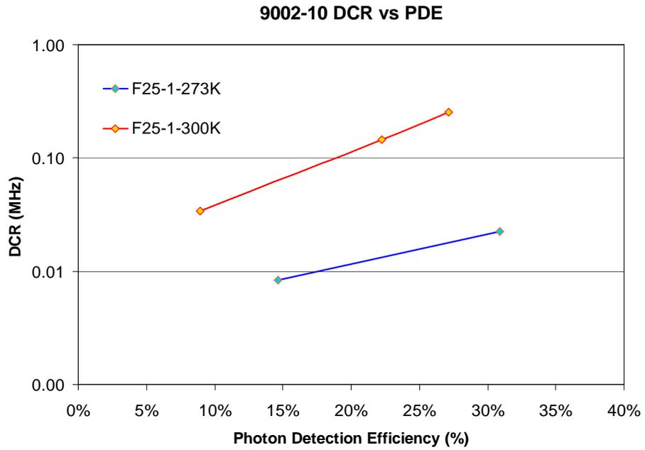
Figure 5 The PDE vs DCR at room temperature and 0°C versus overbias. The PDE was measured at 1.55  $\mu\text{m}$ .
