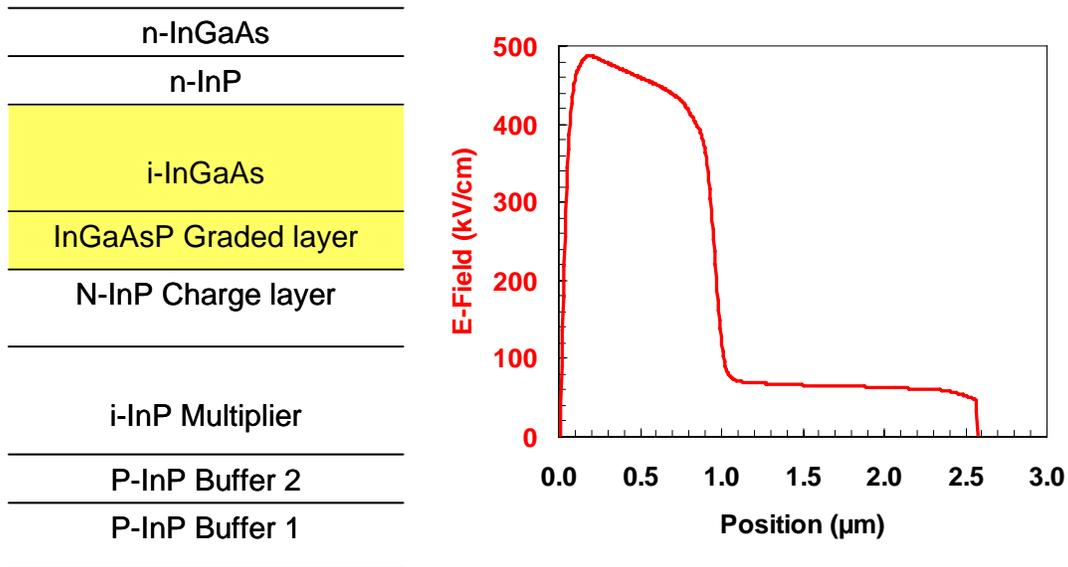
Figure 1 The cross section of the InP/InGaAs Geiger-Mode APD epitaxial stack and its typical electric field profile at operation. The position coordinate starts from the bottom p-i InP interface.
