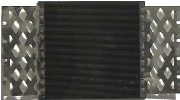
Fig. 7. The CDO-100-IC cell with leads (ICs) attached.
