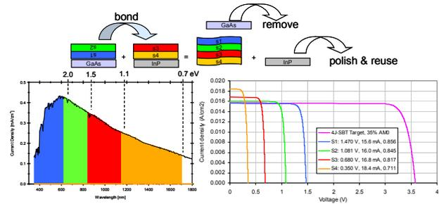
Target parameters:  $V_{OC} \approx 3.6$  V,  $J_{SC} \approx 16$  mA/cm<sup>2</sup>, FF  $\approx 84\%$ , eff. 35% AM0
