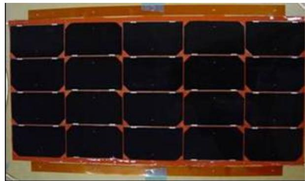
Figure 7. An assembled IBIS coupon.
