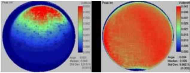
**Figure 8.** Photoluminescence maps of 1 eV metamorphic wafers show recent progress in material quality.
