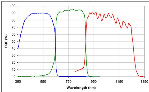
Figure 3. Typical external quantum efficiency characteristics collected on the 3J IMM solar cells shown in Figure 2.
