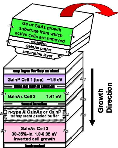
Figure 1. A typical IMM solar cell that is grown in an inverted configuration on a Ge or GaAs substrate. The grown structure is affixed to a handle and the growth substrate removed.
