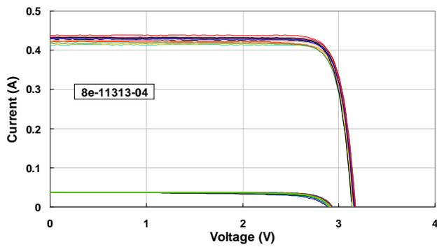
Figure 4. 25 °C LIV characteristics of low concentration IMM cells at 1X AM0 and ~12X AM0 concentration.
