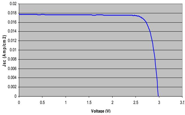
Figure 2. The LIV characteristic of a 1x1 cm<sup>2</sup> 3J IMM cell at 28 °C. This cell was designed for 1 sun AM0 applications and has an AM0 conversion efficiency of 32.6%. The reported efficiency is based on Lear Jet IMM calibration standards.
