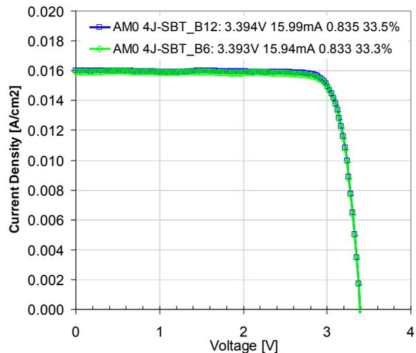
**Figure 12.** The AM0 LIV characteristics of 1x1 cm<sup>2</sup> 4J SBT cells.
