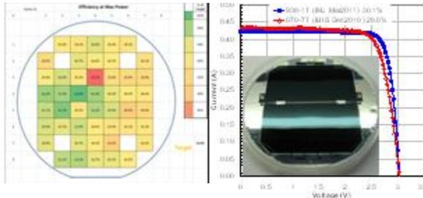
**Figure 9.** A wafer uniformity map of 1x1 cm<sup>2</sup> 3J IMM cells and LIV characteristics of large area 26 cm<sup>2</sup> cells built from similar material.
