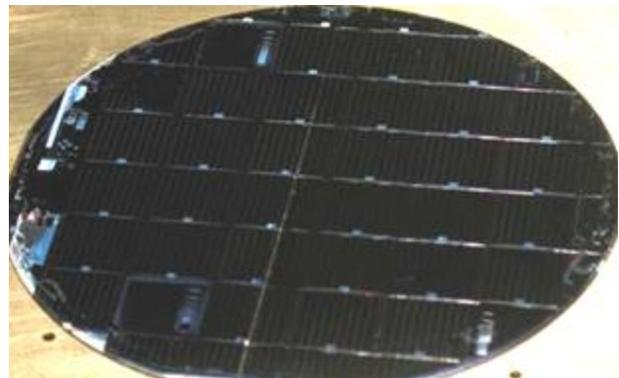
**Figure 11.** A 4J SBT wafer fabricated with 1x1 cm<sup>2</sup> cells.
