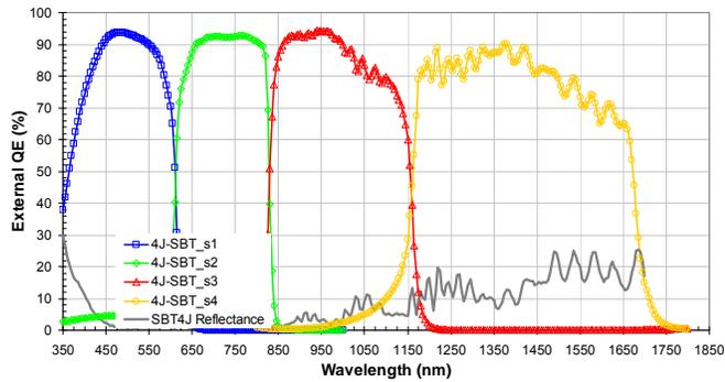
**Figure 13. The external quantum efficiency versus wavelength as measured on a 4J SBT solar cell.**
