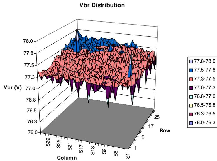
Figure 9. The breakdown voltage characteristics across a Spectrolab 1.06  $\mu\text{m}$  GM-APD array measured at 20  $^{\circ}\text{C}$ .
