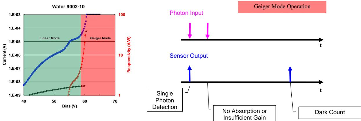
**Figure 1.** Geiger mode operation of an avalanche photodiode.
