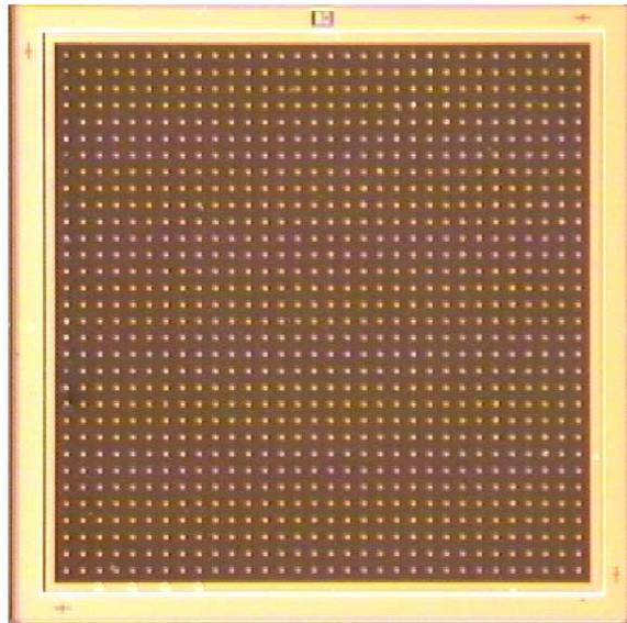
Figure 5. Photograph of a 32 x 32 Gm-APD detector array
