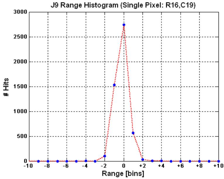
Figure 8. Jitter data collected on a single pixel of a Spectrolab 1.06  $\mu\text{m}$  GM-APD module. Each bin corresponds to 500 ps. After accounting for system jitter, a FWHM of less than 3 bins corresponds to a jitter less than 500 ps.
