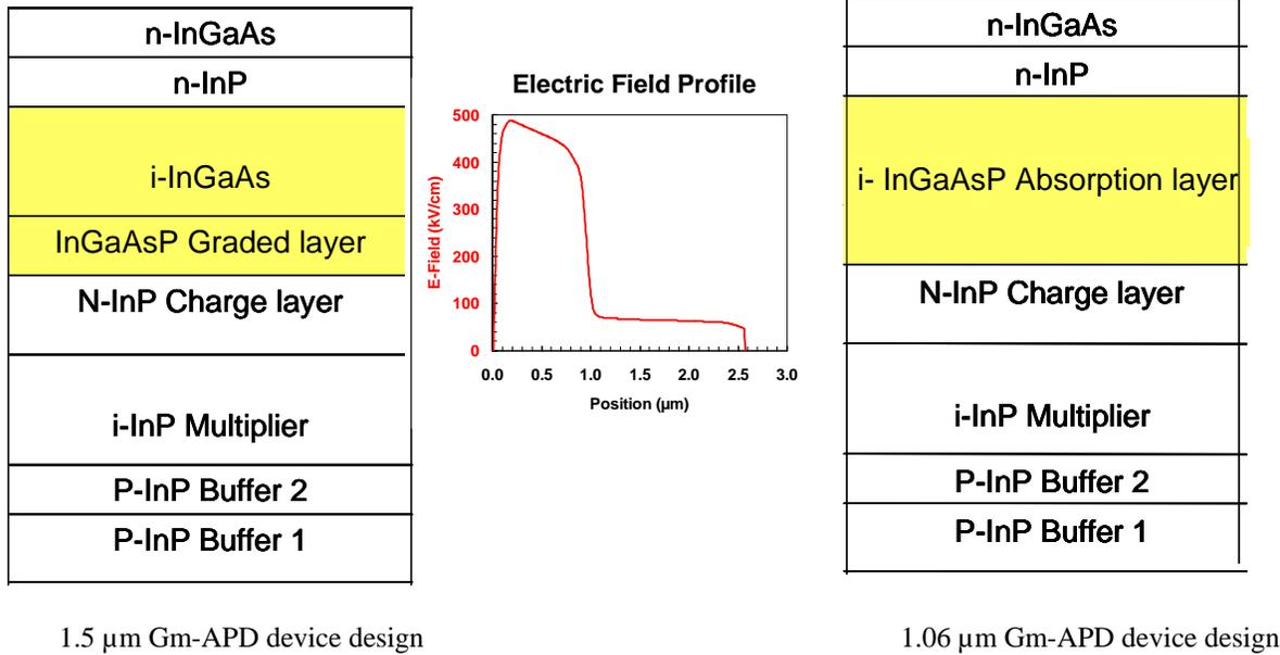
**Figure 2.** Gm-APD device designs and the electric field profile of the designs
