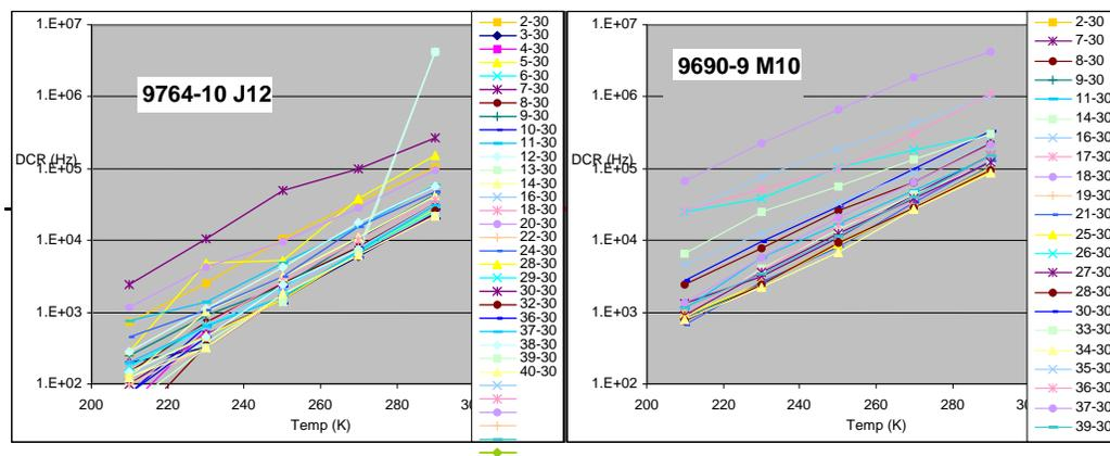
Figure 6. Dark count rate data collected on two recent Spectrolab 32x32 focal plane arrays. All data are taken with a 4 volt overbias on 30  $\mu$ m diameter pixels.
