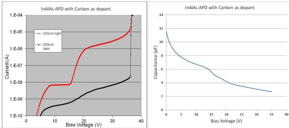
Figure 8 Current voltage characteristics and capacitance voltage characteristics of an InAlAs APD with Carbon as dopant and 200  $\mu\text{m}$  diameter.
