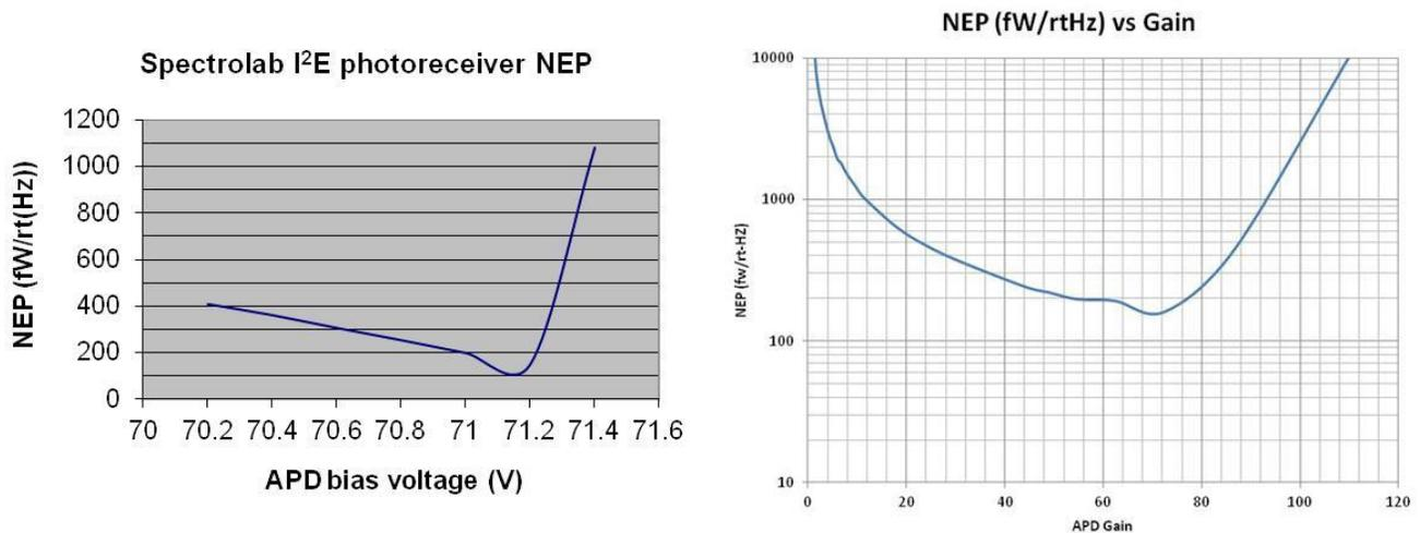
Figure 6 NEPs of photoreceivers build with same GHz TIA and: left, a Gen 2 APD; right, a Gen 3 5 periods I<sup>2</sup>E APDs.
