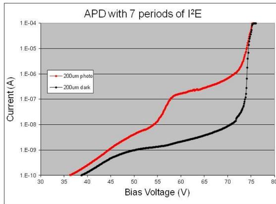
Figure 4 Current voltage characteristics of an APD with 7 periods of  $I^2E$  and 200 $\mu\text{m}$  diameter.
