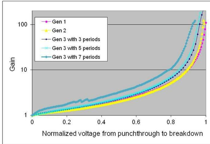
Figure 5 Gain vs. normalized bias of multiple I<sup>2</sup>E APDs.
