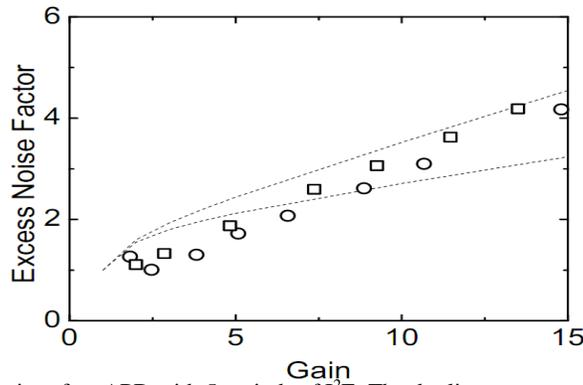
Figure 3 Excess noise of an APD with 5 periods of  $I^2E$ . The dot line corresponds to  $k=0.1$  and  $k=0.15$ .
