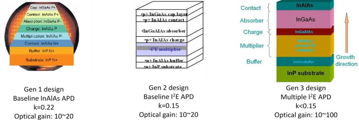
Figure 1 Three generations low noise APDs developed at Spectrolab.
