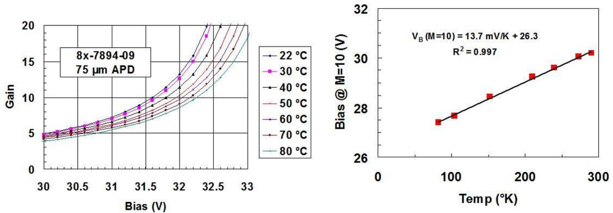
Figure 2 Left: Gain vs. bias voltage of Spectrolab baseline InAlAs APDs. Right: bias voltage@gain=10 vs. temperatures.
