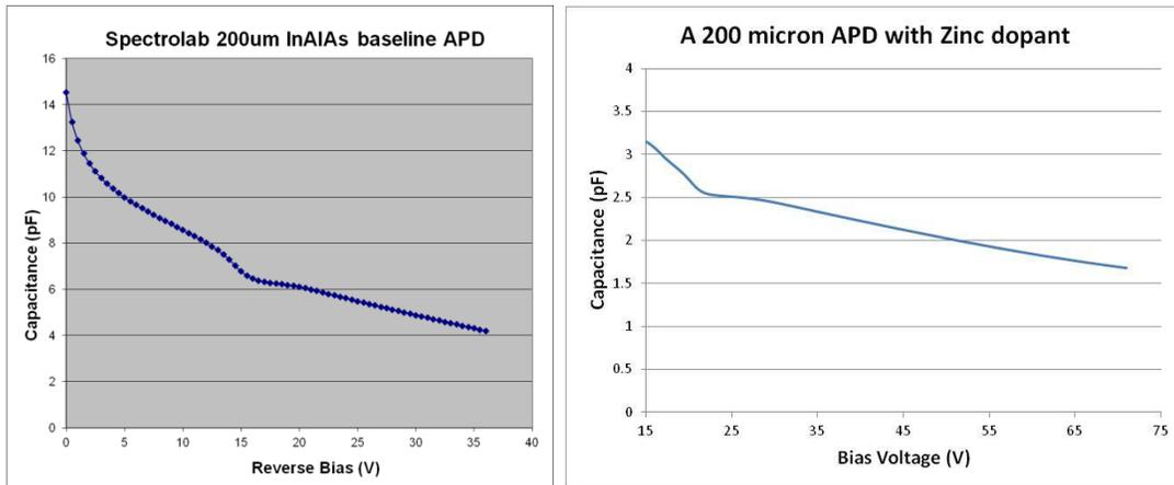
Figure 7 Capacitance voltage characteristics of: left, Gen 1 APD; right, Gen 3 5 periods  $I^2E$  APD with 200  $\mu\text{m}$  diameter.
